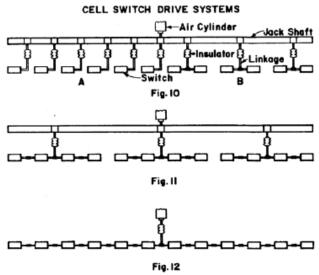
These parameters are largely under the control of the user. Routine maintenance items such as good lubrication of the drive and elimination of backlash from worn parts help prevent insidious contact erosion caused by an unnoticed slowdown in the mechanism speed. Fluctuating air pressure or insufficient air delivery can be corrected by an accumulator or larger air lines.
